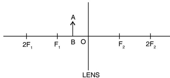
Copy the diagram and by using three standard rays starting from point A, obtain an image of the object AB.
