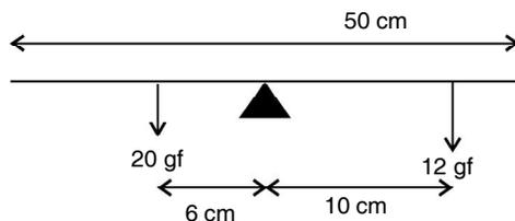
(i) Which of the two forces acting on the rigid rod causes clockwise moment?
