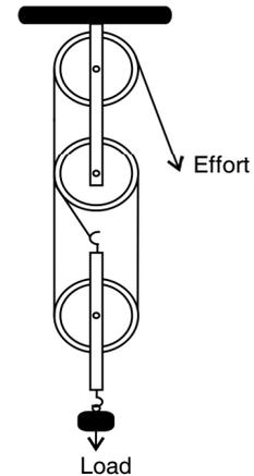
**Ans.** (i) The block and tackle pulley system with velocity ratio 3 is shown below in which the direction of load (L), effort (E) and tension (T) has been marked.
